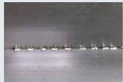
Corner spot welding thickness 0,6 mm
