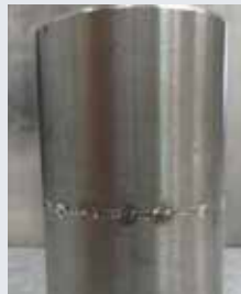
Pipe butt weld Ø 31,75 x 2 mm.
