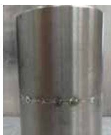
Pipe butt weld Ø 31,75 x 2 mm.
