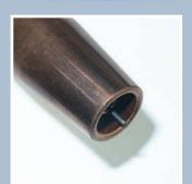
BURN BACK: An optimal wire cutting at the end of welding helps perfect starts.
