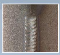
WELDING POSITION: HAC gives an optimal fusion of the bead's edges in short arc welding and to make overhead and vertical up position welding easier.
