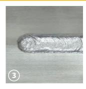
LEVEL 3: A low current ends the welding optimally by filling the crater on weld beads.
