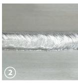
LEVEL 2: The welding current is optimized with the plate thickness and the requested weld.
