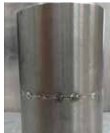
Pipe butt weld Ø 31.75 x 2 mm
