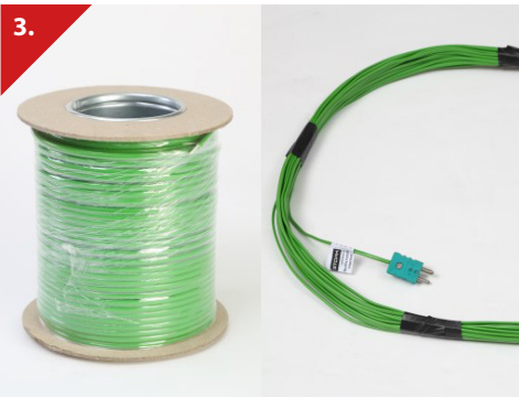
3. Thermocouple Compensating Cable Suitable for use with type K thermocouples where monitoring thermocouples, in addition to the control thermocouples, are required for temperature monitoring purposes. Available in 30m lengths complete with type K thermocouple plug and socket or in 100m rolls without plug and socket (plugs and sockets can be supplied separately as required). Stork reference & description: 34000 - 30m compensating cable c/w type K thermocouple plug and socket 504-062 - 100m roll of compensating cable without thermocouple plug or socket (green) 304-065 - 100m roll of compensating cable without thermocouple plug or socket (red)
