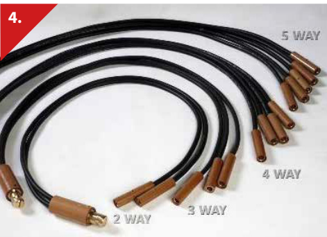
4. Splitter Cables For use with triple cable sets. Splitters are used where the operator needs to connect multiple heating elements, in parallel, to triple cable sets to enable the control of multiple heating elements. this enables the heating elements to be grouped to a single control output from a heat treatment unit to allow accurate zonal temperature control. Stork reference & description: 32001 2 Way splitter 32002 3 Way splitter 32003 4 Way splitter 32004 5 Way splitter
