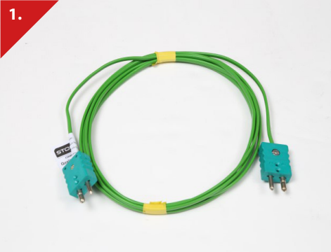
1. Compensating Cable Link Cables To link controller/programmer thermocouple input to the recorder input. Stork reference & description: 34013 - 3m jumper' compensating lead fitted with two type K thermocouple plugs
