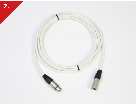
2. Compensating Cable Control Leads To connect separate, external controller/programmer unit's output to power source control input. Stork reference & description: 33009 - 3m 3-core, programmer/contractor control lead
